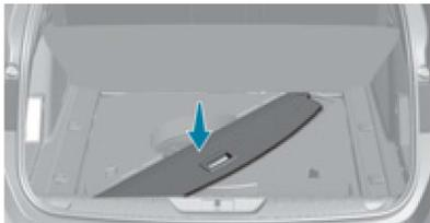
A recess in the floor well, under the boot carpet, allows the luggage cover to be stowed diagonally.
