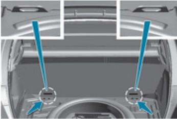
A ring **B** located in the boot (indicated by a marking), referred to as the **TOP TETHER** for fixing the upper strap.
