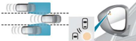
This driving assistance system warns the driver of the presence of another vehicle in the blind spot angle of their vehicle (areas masked from the driver's field of vision), as soon as this presents a potential danger.
