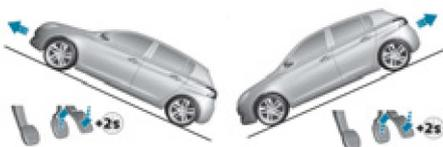
**On an ascending slope, with the vehicle stationary, the vehicle is held for a momentarily when you release the brake pedal.**
