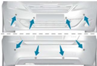
This system indicates the proximity of an obstacle (examples: pedestrian, vehicle, tree, gate) which comes within the field of detection of sensors located in the bumper.
