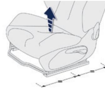
**Passenger seat adjusted to the intermediate longitudinal and highest position.**
