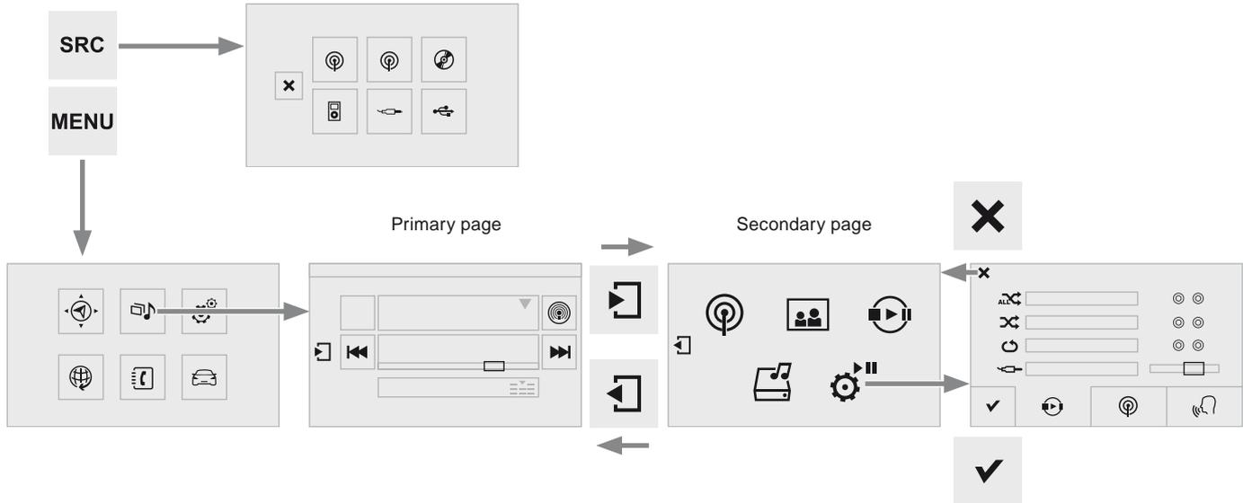
Short-cuts: using the touch buttons in the upper band of the touch screen, it is possible to go directly to the selection of audio source, the list of stations (or titles, depending on the source).
