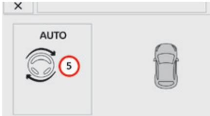
The assisted parking manoeuvre is in progress. Without exceeding 5 mph (8 km/h), continue the manoeuvres following the information given by the "parking assistance" system, until the end of manoeuvre message is displayed. The indicator lamp in the control goes off, accompanied by an audible signal.
