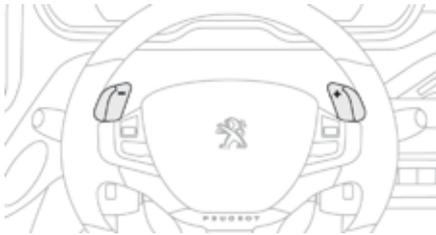
This selective gear change mode enables you to overtake, for example, while still remaining in automatic mode.
