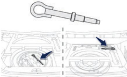
The towing eye is installed in the boot under the floor.
