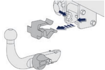
Remove the protective blanking plug from the carrier and check the condition of the fixing system. If necessary, clean the carrier with a brush or clean cloth.
