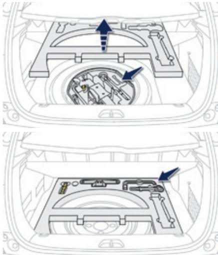
The tools are installed in the boot under the floor.
