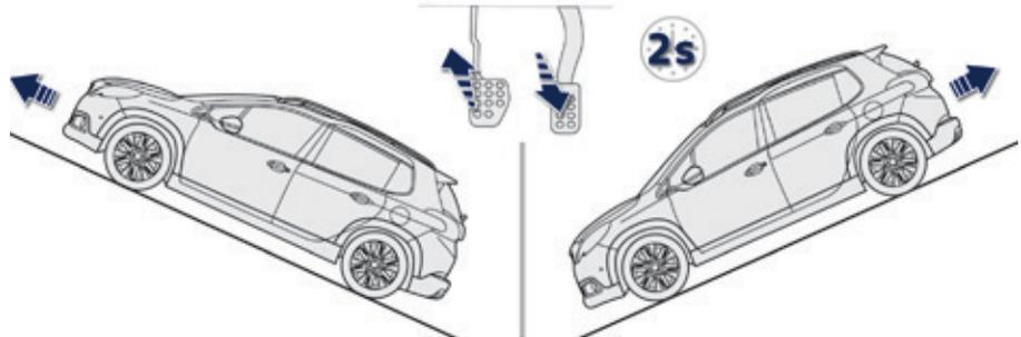
**On an ascending slope, the vehicle is held for a brief moment when you release the brake pedal:**
