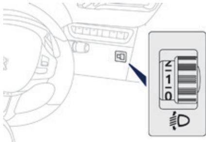
To avoid causing a nuisance to other road users, the headlamp beams should be adjusted according to the load in the vehicle.
