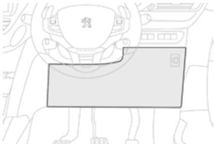
The fusebox is placed in the lower dashboard (right-hand side).
