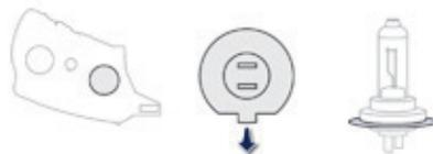
To reassemble, carry out these operations in reverse order, positioning the alignment lug at the bottom.
