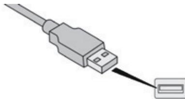
Connect a USB memory stick to the USB port or connect a USB device to the USB port using a suitable cable (not supplied).
