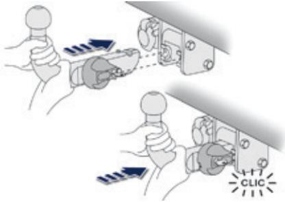
Take the towball in both hands; insert the end of the towball into the carrier, then, to ensure that it has correctly locked in place, pull firmly down on the ball end of the towball. The locking wheel automatically turns a quarter of a turn anti-clockwise, making a perceptible click; take care to keep your hands clear.
