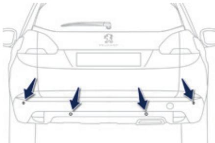
This system indicates the proximity of an obstacle (pedestrian, vehicle, tree, gate, etc.) which comes within the field of detection of sensors located in the bumper. Certain types of obstacle (stake, roadworks cone, etc.) detected initially will no longer be detected at the end of the manoeuvre, if they are located in blind spots in the sensors' field of detection.
