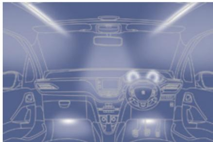
At night, interior mood light emitting diodes - LEDs (courtesy lamp, instrument panel, footwells, back-lit roof lining, panoramic glazed sunroof\*...) come on automatically when the sidelamps are switched on.
