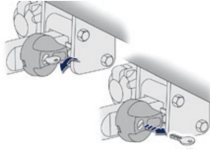
Check that the towball has correctly locked in place (position **A**).
