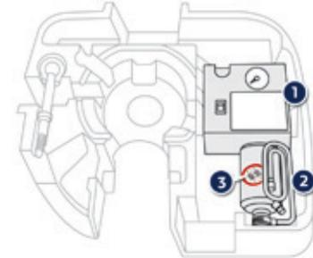
1. 12 V compressor, with integral pressure gauge.
