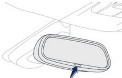
This system automatically and progressively changes between the day and night uses by means of a sensor, which measures the light from the rear of the vehicle.
