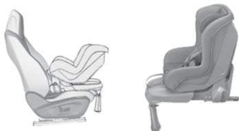
Installed "rearward facing" using an ISOFIX base which is attached to the rings **A**.
