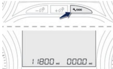
With the trip mileage displayed, press this button for a few seconds.
