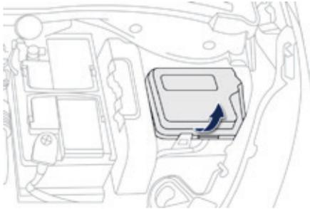
The fusebox is placed in the engine compartment near the battery (left-hand side).
