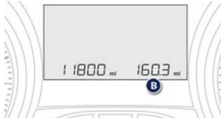
System that measures the distance travelled (daily, for example) since it was last reset by the driver. The trip recorder is displayed in zone **B** of the instrument panel screen.
