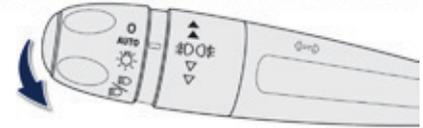
Side markers for the vehicle by illumination of the sidelamps on the traffic side only.
