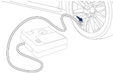
To check and if necessary adjust the tyre pressures.
