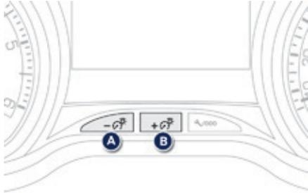
With the headlamps on, press button **B** to increase the brightness of the instruments and controls and the interior mood lighting or button **A** to reduce it. As soon as the lighting reaches the required level of brightness, release the button.
