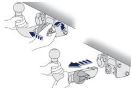
Grasp the towball firmly with one hand; with the other hand, press and turn the locking wheel clockwise as far as it will go.
