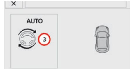
The assisted exit from parking manoeuvre is in progress. Without exceeding 5 mph (8 km/h), continue the manoeuvres following the information given by the "parking assistance" system, until the end of manoeuvre message is displayed. The manoeuvre is complete once the front wheels of the vehicle are out of the parking space. The indicator lamp in the control goes off, accompanied by an audible signal.
