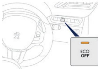
In the event of a fault with the system, the "ECO OFF" switch warning lamp flashes then comes on continuously. Have it checked by a PEUGEOT dealer or a qualified workshop. In the event of a fault in STOP mode, the vehicle may stall. All of the warning lamps come on. It is then necessary to switch off the ignition and start the engine again using the key.
