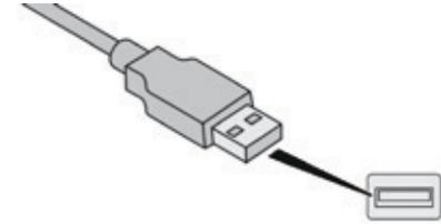
Connect the Apple® player to the USB port using a suitable cable (not supplied).
