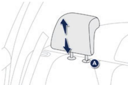
These have one position for use (up) and a stowed position (down). They can be removed and are interchangeable side to side.
