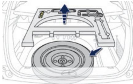
The spare wheel is installed in the boot under the floor.
