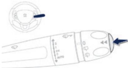
☞ Press the button on the end of the **wiper control stalk** to display the various tabs in succession.
