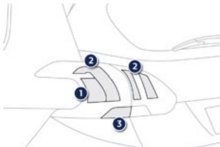
1. Brake lamps (P21W) (light-emitting diodes-LEDs).
