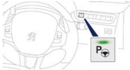
With the vehicle stationary, to activate the Park Assist system:
