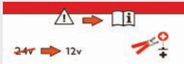
If this label is present, it is essential to use only a 12 V charger, to avoid causing irreversible damage to the electrical components related to the Stop & Start system.
