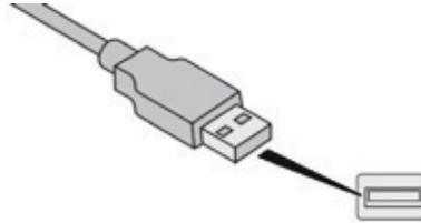
Connect the Apple® player to the USB port using a suitable cable (not supplied).
