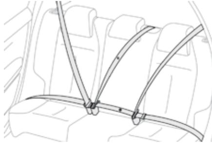
The rear seats are each fitted with a three-point seat belt.
