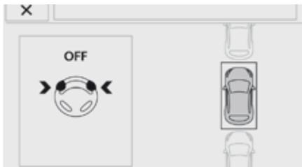
The driver takes back control of the vehicle's steering.
