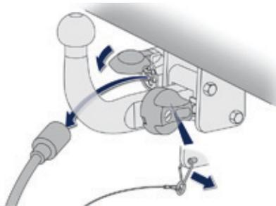
Disconnect the trailer harness from the socket on the carrier.
