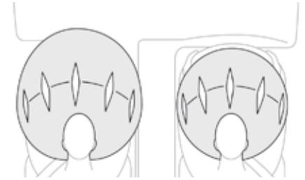
System which protects the driver and front passenger in the event of a serious front impact, in order to limit the risk of injury to the head and thorax.
