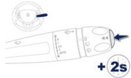
☞ When the trip required is displayed, press the control for more than two seconds or use the left hand thumb wheel of the steering mounted controls.
