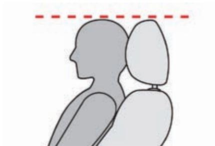
! The head restraint has a frame with notches which prevent it from lowering; this is a safety device in case of impact. **The adjustment is correct when the upper edge of the head restraint is level with the top of the head.** Never drive with the head restraints removed; they must be in place and adjusted correctly.
