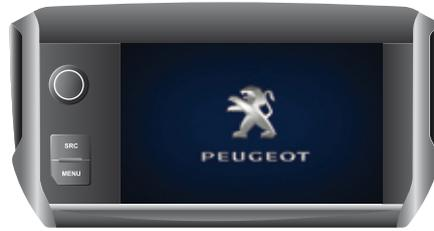
**i** In very hot conditions, the system may go into stand-by (screen and sound completely off) for a minimum period of 5 minutes.
