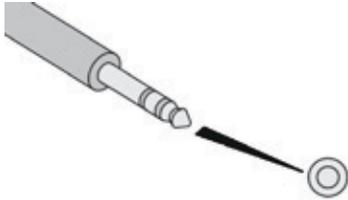
Connect the portable device (MP3 player...) to the Jack auxiliary socket using an audio cable (not supplied).
