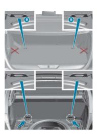
A ring **B** located in the boot (indicated by a marking), referred to as the **TOP TETHER** for fixing the upper strap.
