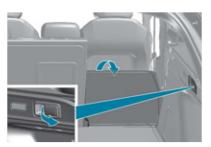
Pull the control from inside the boot, the seat backrest folds onto the cushion.
