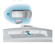
With the electronic key on your person in the recognition zone A, press the opening control then raise the tailgate.
