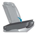
Pull the control 1 forwards, the seat backrest folds onto the cushion.
